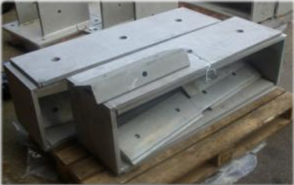
Brackets produced for flood defence work
